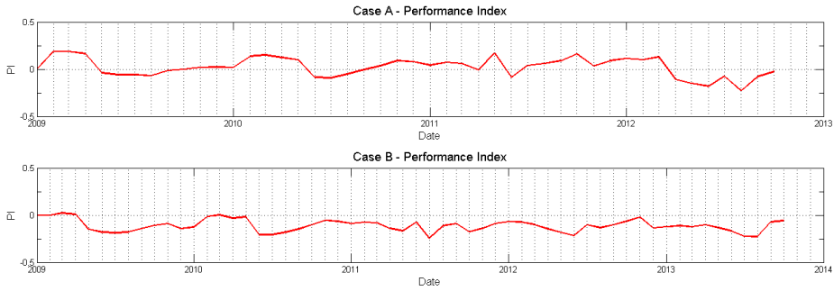
Fig. 6. Power Curve Monitoring with the Performance Index.
