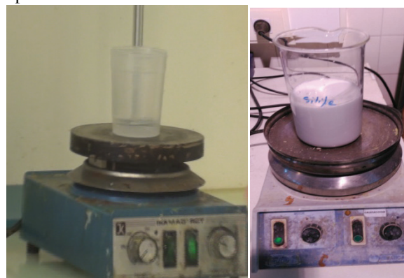
Fig. 3. Hydrolysis with HCl (left). Stirring suspension with quartz (right).
