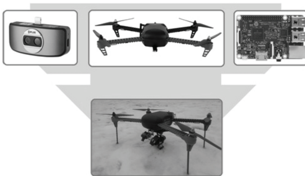
Fig. 2. Quadcopter infrared vision platform assembly.
