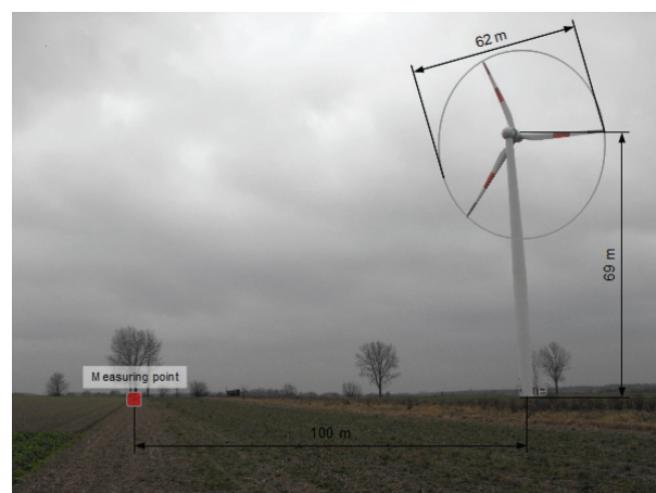
Fig. 2. Location of the infrasound noise level measuring point at the synchronous type turbine.
