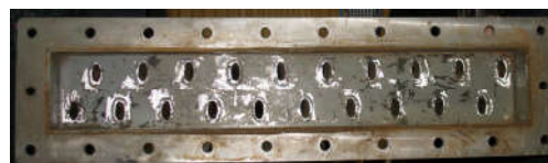
Fig. 12. A view of sieve plate and its connection with heat exchanger header
