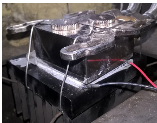
Figure 7. Cooling of the TEG using the water heat exchanger.
