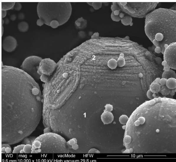
Figure 9. SEM microphotograph of magnetic residues after demagnetization process-microphotograph 2
