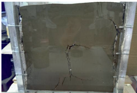
Figure 1. Evaporating clay slurry showing crack development below the surface in the clay body.
