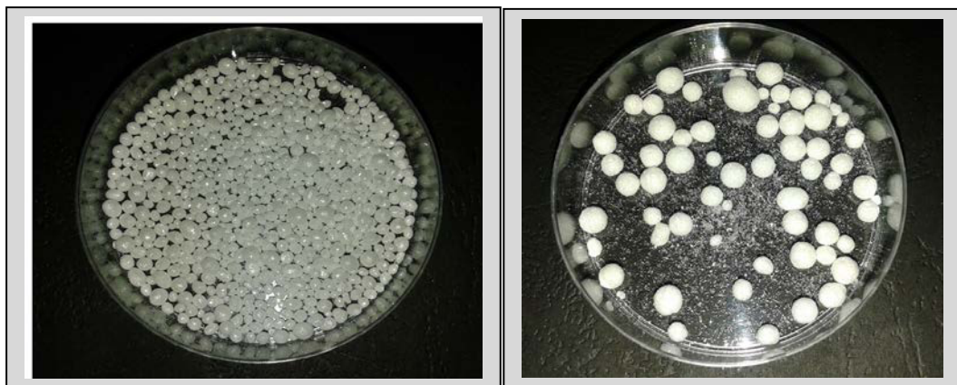
Figure 1. Acetylsalicylic acid crystals agglomerates obtained for the solid-to-liquid ratio of 2 g/10 ml (left) 1 g/10 ml (right) as well as 1.8 ml (left) and 0.8 ml (right) of carbon tetrachloride as the bridging liquid.
