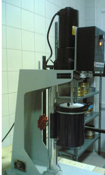
Figure 2. A stirred ball mill used in grinding tests.
